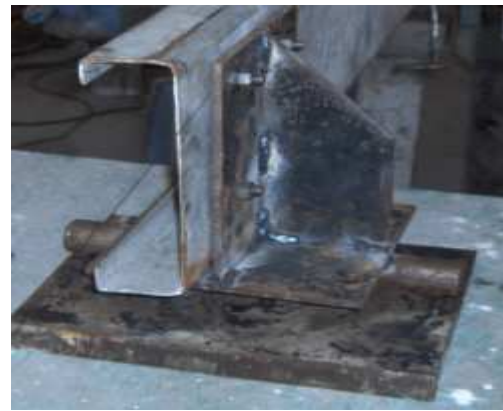
Fig. 3 End Connection Details
