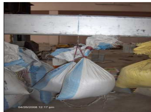
Fig. 4 Loading Arrangement.(Sand Bags)
